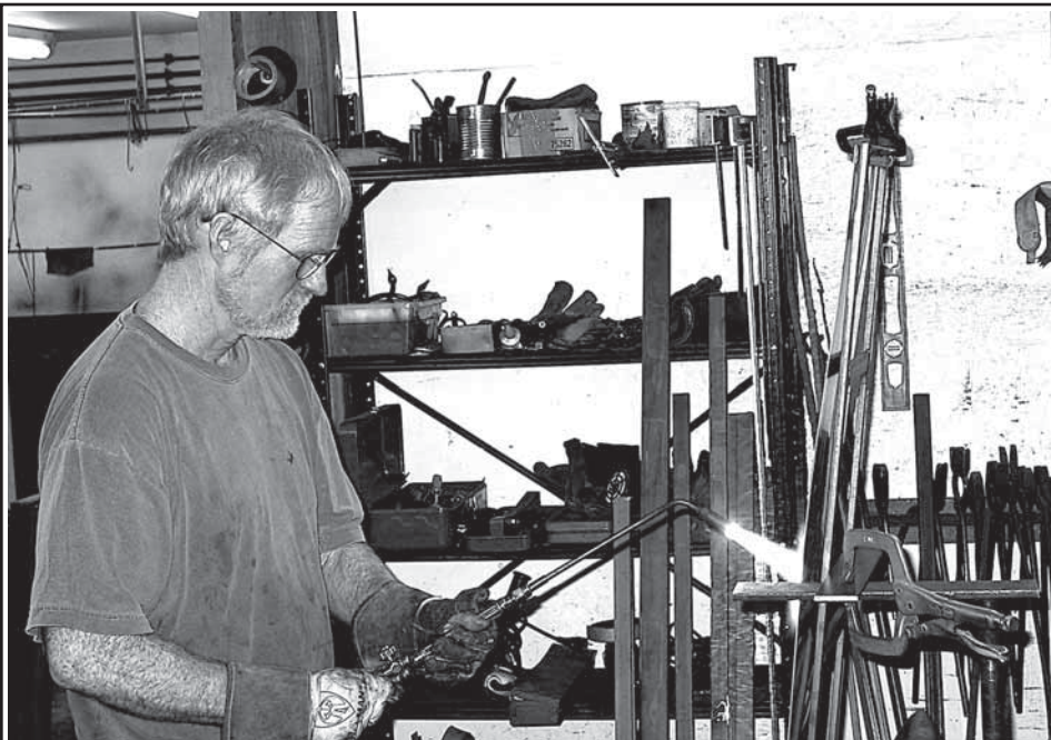
photo by Charles Sutton Working on a set of custom-made fireplace doors, Payne Junker uses a torch to bring out the colors in the metal.
